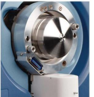
Figure 2. SelexION+ interfaced to SCIEX 6500+ Triple Quad
